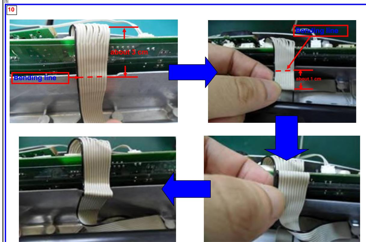
11. Insert the bended loadcell cable into the space between film and bottom.
