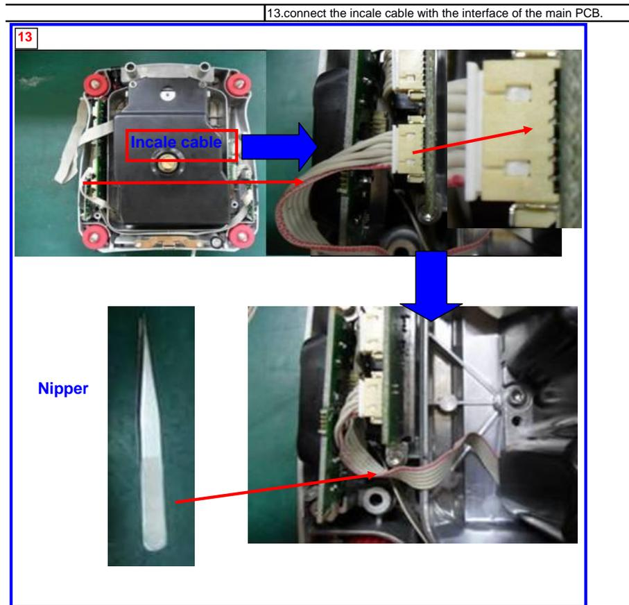
Load-cell cable routing – Draftshield models:
