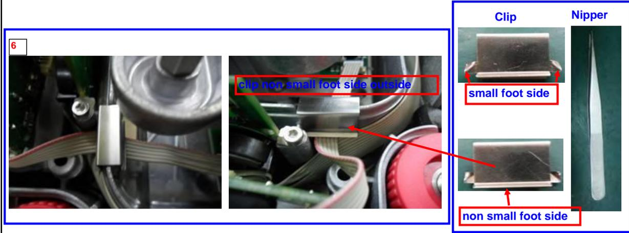
7. Put the cable into the slot using nipper and make sure the cable not cover the screw hole
