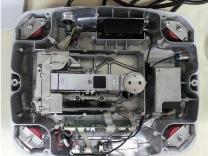
**3.3 REPLACING THE LOAD CELL (not 12001, 24001 and 35001)**
