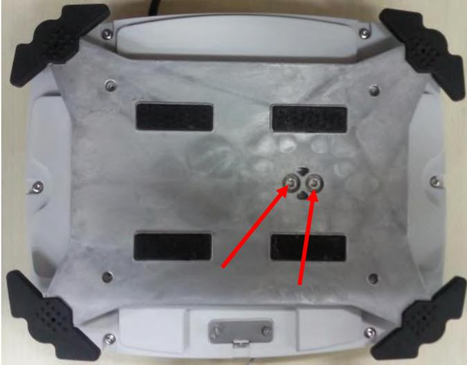
3. Remove the 7 screws that hold the Top Housing to the Base.
