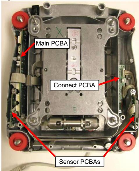
2. Remove IR Sensor PCBAs
