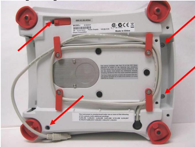
3. Turn the base back on its feet and remove the Top Housing. Lay the Top Housing alongside so that the Bubble Level Light wiring can be disconnected.
