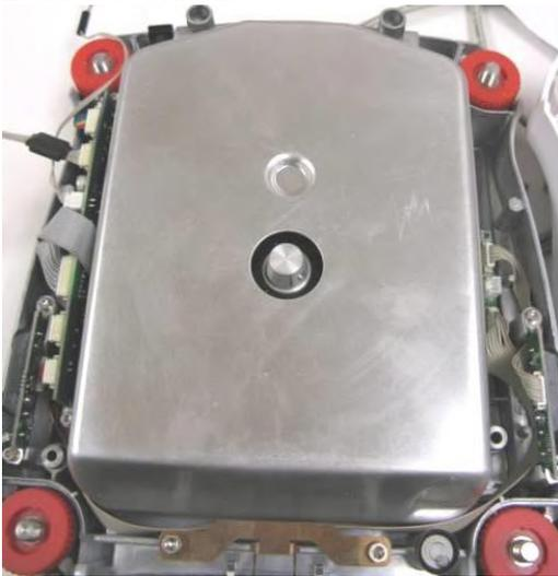
3. Disconnect the two Load Cell connections at the Main PCB.
