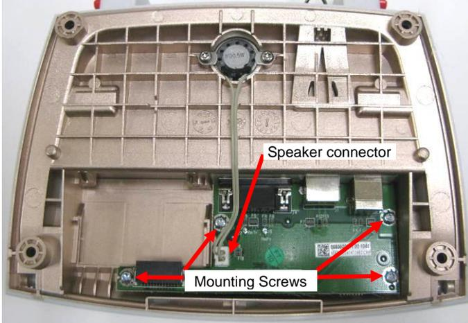
4. To remove the speaker remove the 2 screws and lift out.
