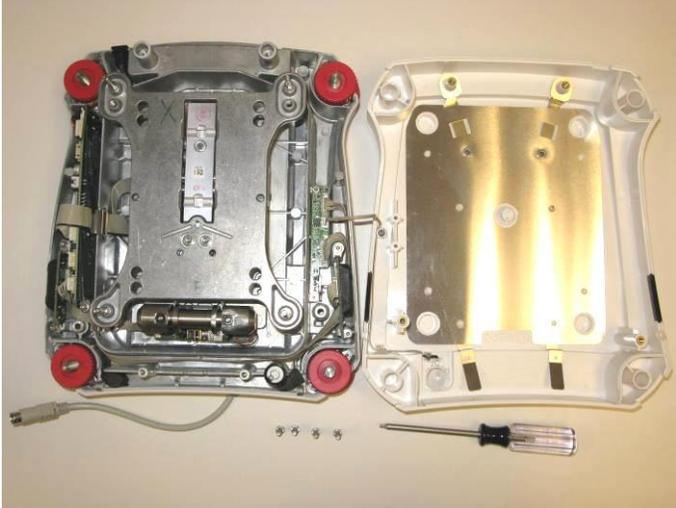
4. Disconnect the Bubble Level Light wiring by pulling up on the connector.
