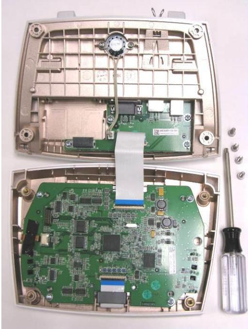
4. Disconnect the ribbon cable connecting the two assemblies. Using a finger nail or a thin screw driver blade rotate the black cable-lock on the connector 90° so that it is perpendicular to the cable.
