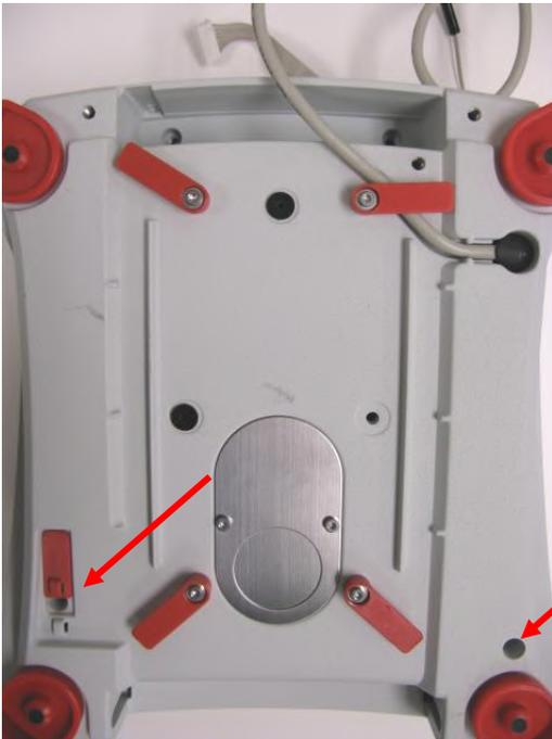
8. Turn the Module over. Remove the Top Housing being careful to route the Light Cable and Motor Cables (if equipped) through the holes in the Upper Housing.
