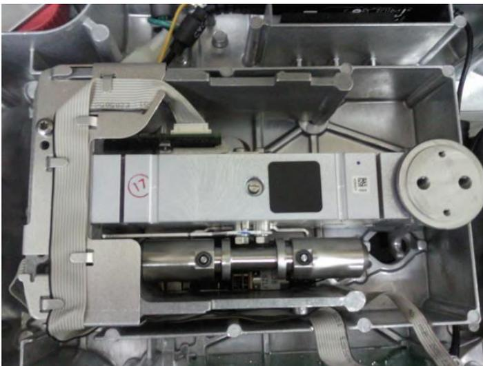
4. Remove all cables connecting the load cell to the PCB and lift the load cell out from the housing.
