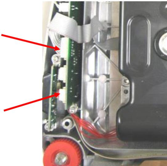
4. Remove the Load Cell –remove the 4 load cell screws from the bottom housing. Lift the Load Cell Module from the Base. Do not lift by the Pan Support Cone or the cables.
