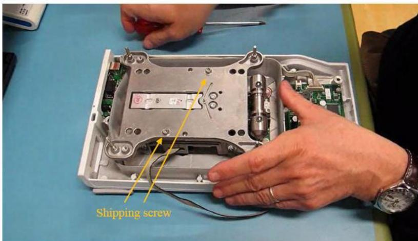
2. Start by removing the screw on your left side. Please pay attention to not shift the spider from its position during this procedure. Follow by removing the screw on the right side.
