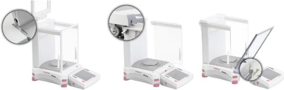
4. Remove the Platform, Sub-Platform, Support Caps and Wind Ring as required.
